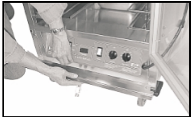
To remove trough: remove thumbscrews; drop trough down and pull forward.
