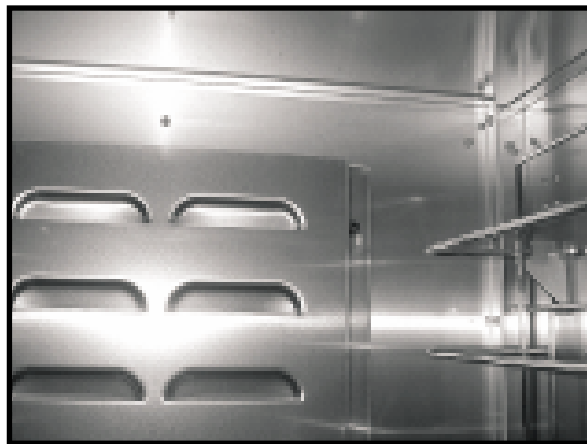
Grasp air tunnel and lift up and off.
