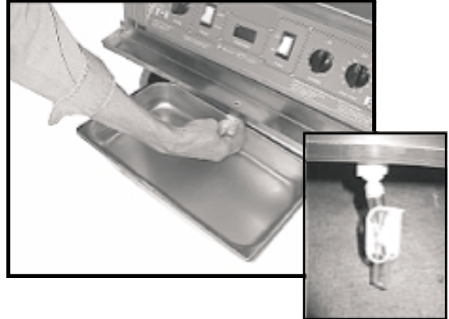
Close by pushing front of clamp inward.
